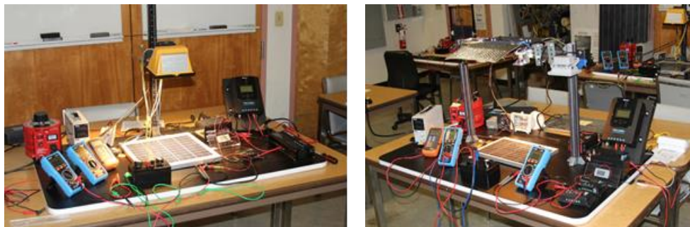
Fig. 2. Lab station 3 (left) and 4 (right) with different illumination systems for characterizing solar modules, for studying elements of balance-of-system and for designing PV autonomous systems
