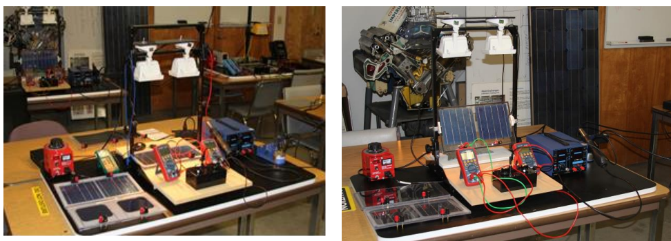
Fig.1. Lab station 1 (left) for studying fundamentals of photovoltaic energy conversion and the solar cells and lab station 2 (right) with additional opportunity to do angular measurements and to study bifacial SCs
