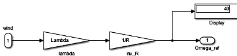
4-rasm. MPPT blokining ichki tuzilishi
