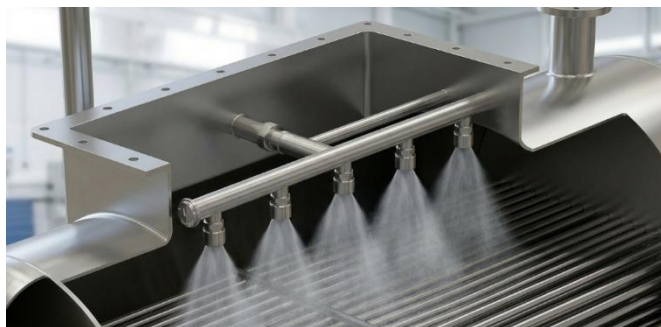
2-rasm. Bug' oqimi bilan bir tarafga yo'nalgan suv sepish jarayoni Figure 2. The process of spraying water in the same direction as the steam flow
