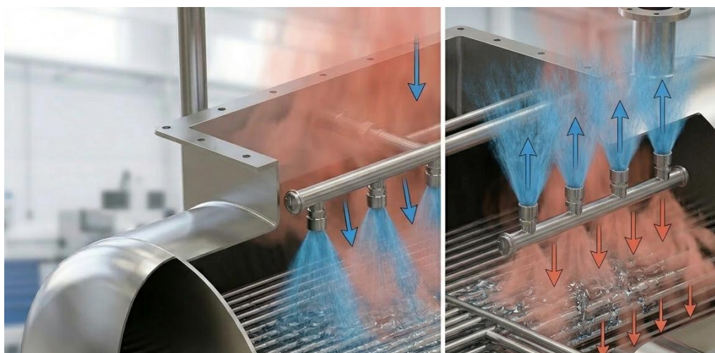
3-rasm. Bug' oqimi bilan bir tarafga va qarama-qarshi tarafga yo'nalgan suv sepish jarayonlari Figure 3. Water spraying processes directed co-currently and counter-currently with the steam flow
